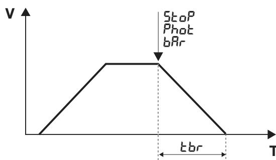
The intervention of the safety input causes an immediate slowing of the gate, the time in which the gate switches from standard speed to a complete stop is adjustable through the TBR value and must respect the values indicated in Table 1.
